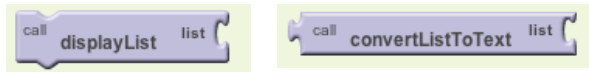
Figure 21-14. The call on the right returns a value and so must be plugged into something
