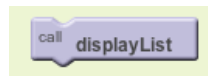
Figure 21-5. A call block appears in “My Definitions” when you define a procedure
